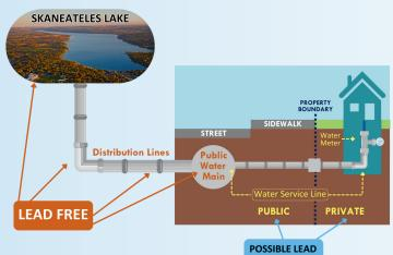
The lead detected in some samples is introduced when the water leaving the City's water mains travels through pipes connecting older homes to the City's water system or, alternatively, when it passes through plumbing fixtures in the home. The Syracuse Department of Water (the "Department") continues to comply with EPA guidelines regarding lead service lines and is working in conjunction with the New York State and Onondaga County Health Departments to address lead concerns.
