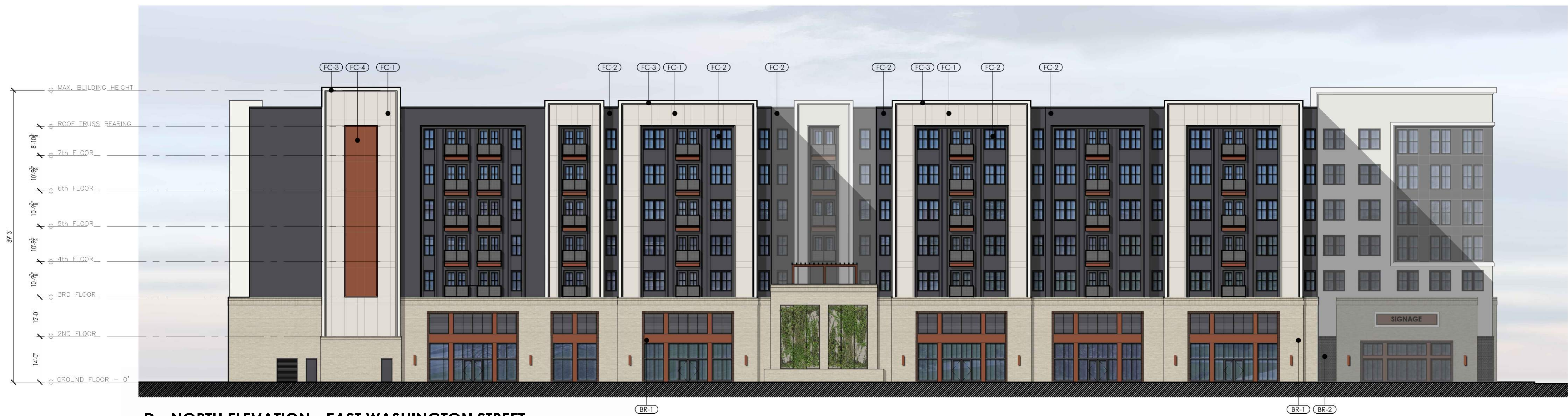
D - NORTH ELEVATION - EAST WASHINGTON STREET
