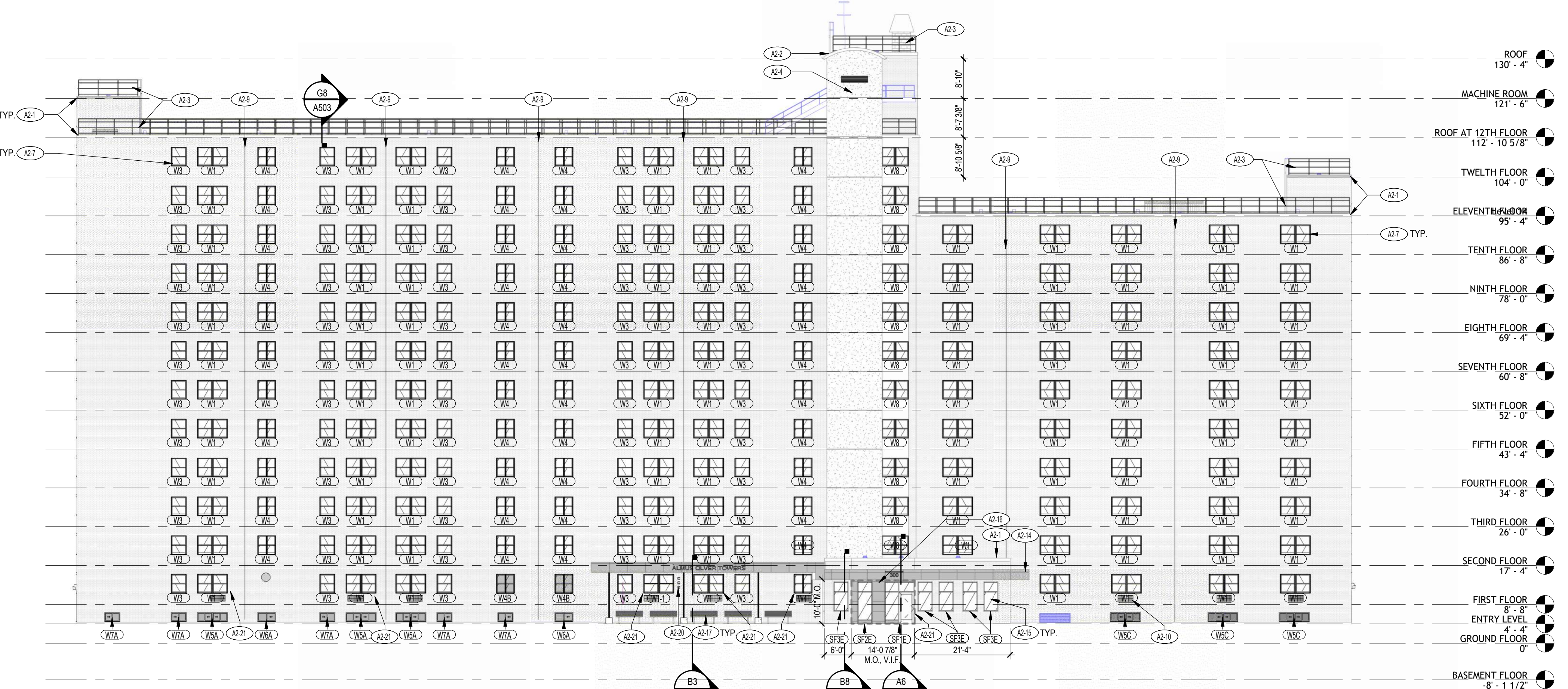
A1 NORTH RENOVATION EXTERIOR ELEVATION 1/16" = 1'-0"
