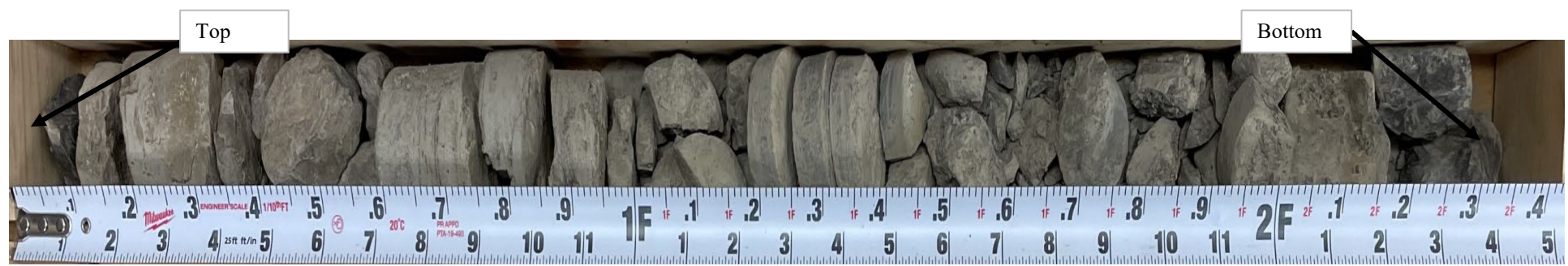
Photograph 1 Boring: B-1A Run 1 Depth 4.5' - 9.5' See Photographs Nos. 2 and 3 for detailed views.
