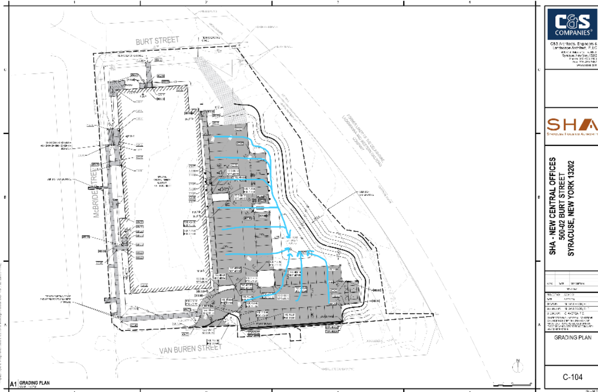
Figure 2: Grading plan annotated to show proposed sheet flow from parking lot area to infiltration basin.
